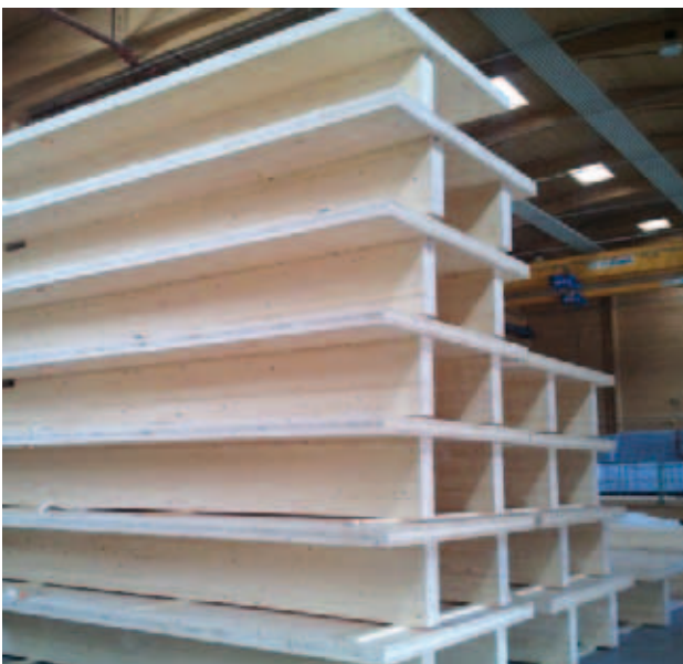
Finished rib elements, ready for transport
