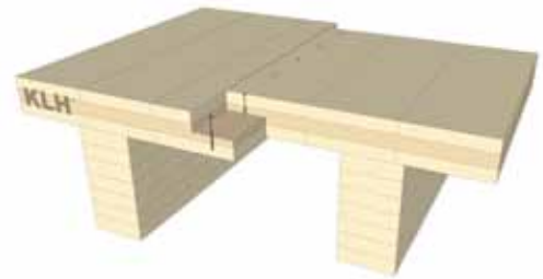
Fig. 6: Element connection with screw-connected stepped joint
