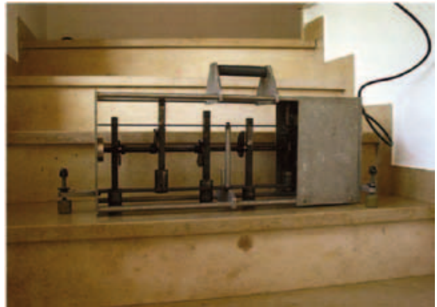
Fig. 20 – Standard impact machine as it is used in determining impact sound levels [7.14]
